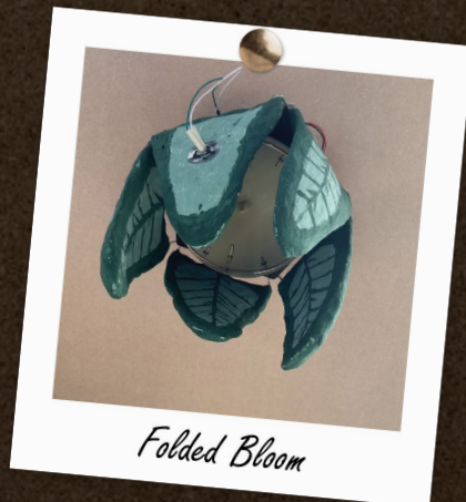
Figure 7. Folded Bloom – Bloom in a closed state in the night. You can see the electronics for the light leaf on the back.
