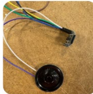
15: Connect the speaker and DF Player to the ESP32
